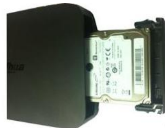
③ Put the HDD into the device
